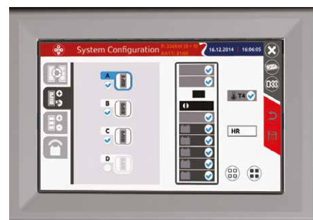
MPW LCD Touch screen: customer oriented UPS configuration and monitoring.
